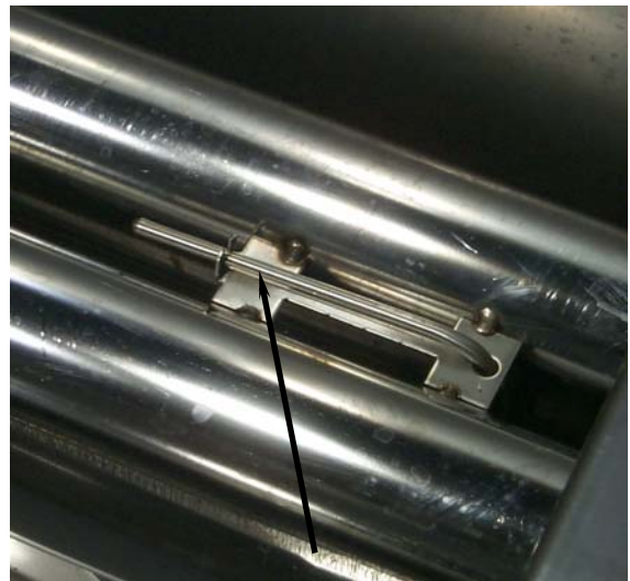
Electronic thermostat probe in frypot (arrow).
